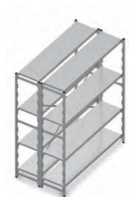
The double shelving unit With back-to-back assembly, you can increase the usable depth of the section. Because the uprights are bolted to each other, there is one less cross brace than with the basic set-up.
